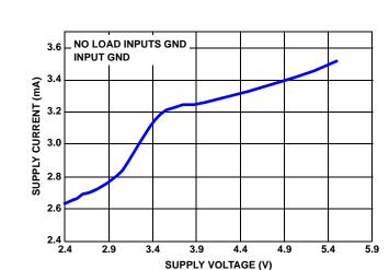
FIGURE 18. SUPPLY CURRENT vs. SUPPLY VOLTAGE
