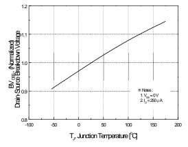
Figure 7. Breakdown Voltage Variation vs. Temperature
