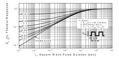
Figure 11. Transient Thermal Response Curve
