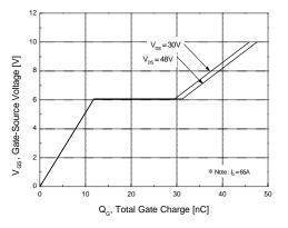
Figure 6. Gate Charge Characteristics
