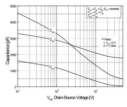
Figure 5. Capacitance Characteristics
