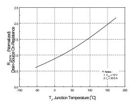
Figure 8. On-Resistance Variation vs. Temperature
