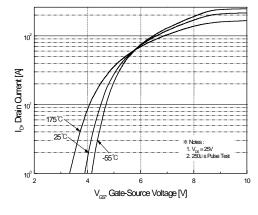
Figure 2. Transfer Characteristics
