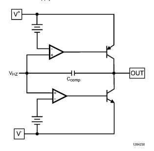
FIGURE 7. Simplified Output Stage Block Diagram
