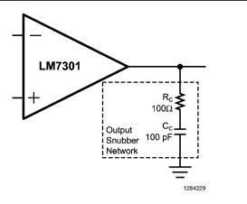
FIGURE 8. Non-dissipating Snubber Network to Reduce Gain Peaking
