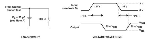
NOTES: A. C<sub>L</sub> includes probe and jig capacitance.
