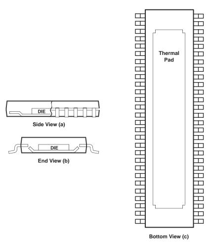
Figure 13. Views of Thermally Enhanced DCA Package
