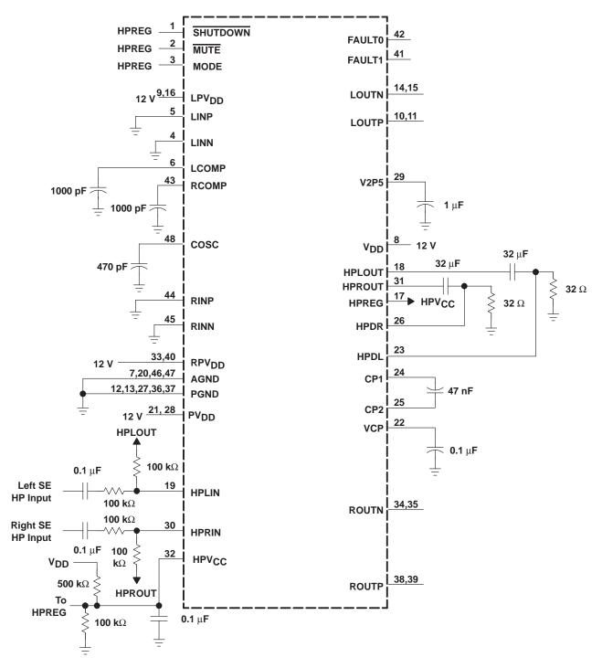
Figure 3. Headphone Test Circuit
