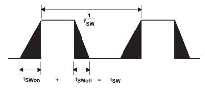
Figure 10. Output Switching Losses
