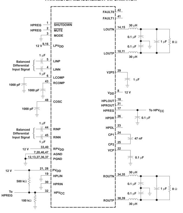
Figure 2. 12-V, 8- $\Omega$  Test Circuit
