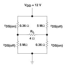
Figure 9. Output Transistor Simplification for Conduction Loss Calculation
