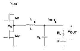
Figure 5. Half-Bridge Class-D Output Stage
