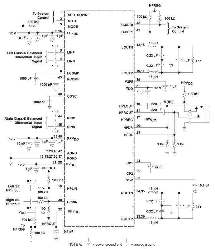
Figure 4. TPA032D04 Typical Configuration Application Circuit
