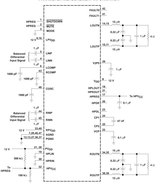
Figure 1. 12-V, 4- $\Omega$  Test Circuit
