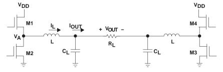
Figure 8. H-Bridge Class-D Output Stage
