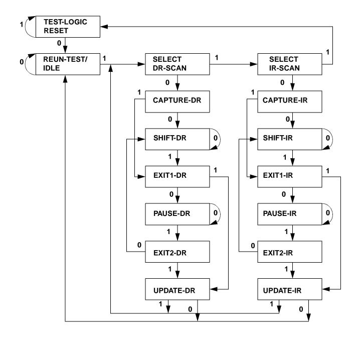
Figure 1. TAP Controller State Diagram<sup>[10]</sup>
