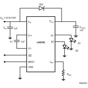
M2792 Current Regulated Switched Capacitor LED Driver with Analog Brightness Contro
