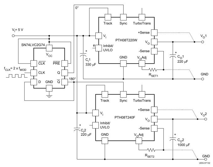
Figure 29. Smart Sync Schematic
