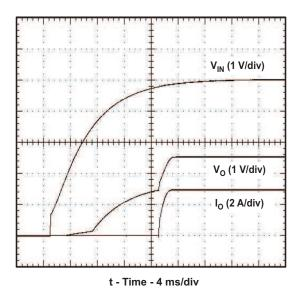
Figure 35. Prebias Startup Waveforms
