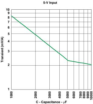
Figure 14. Capacitor Type B, 1000 < C(μF)×ESR(mΩ) ≤ 5000 (e.g. Polymer-Tantalum)
