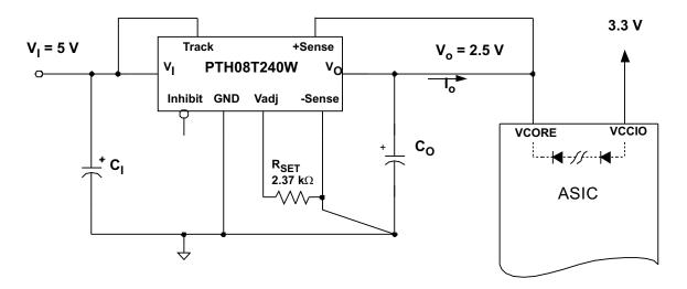
Figure 34. PreBias Startup Application Circuit
