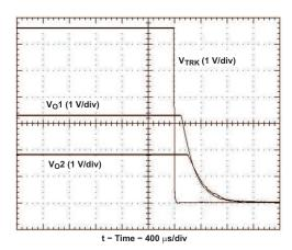
Figure 33. Simultaneous Power Down With Auto-Track Control
