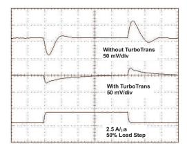
Figure 23. Typical TurboTrans Waveforms (5-V Input)
