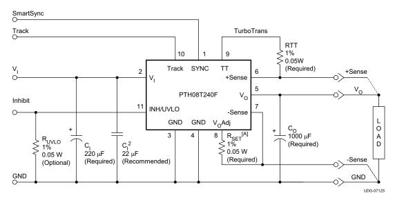
A. R<sub>SET</sub> required to set the output voltage to a value higher than 0.69 V. See *Electrical Characteristics* table.
