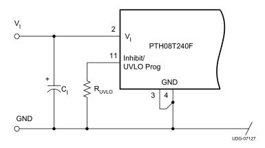
Figure 24. Undervoltage Lockout Adjustment Resistor Placement
