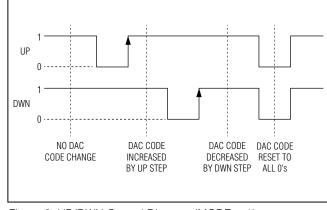
Figure 3. UP/DWN Control Diagram (MODE = 1)
