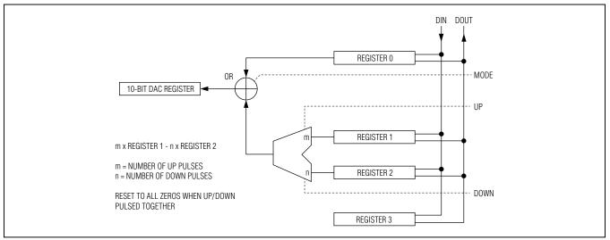
Figure 1. Register Configuration Diagram
