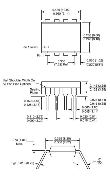
NOTE: 1. ALL DIMENSIONS IN INCHES (IN PARENTHESES IN MILLIMETERS) 2. PACKAGE DIMENSIONS EXCLUDE MOLDING FLASH
