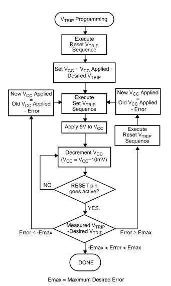
FIGURE 4. VTRIP PROGRAMMING SEQUENCE
