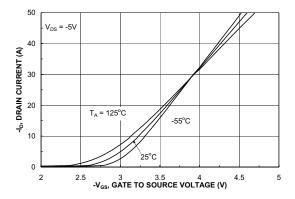
Figure 5. Transfer Characteristics.
