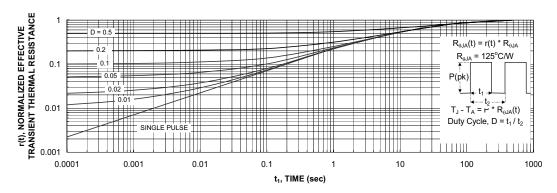
Figure 11. Transient Thermal Response Curve.
