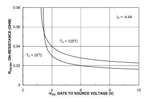
Figure 4. On-Resistance Variation with Gate-to-Source Voltage.
