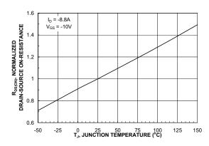
Figure 3. On-Resistance Variation with Temperature.
