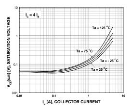
Figure 6. Saturation Voltage (R-Grade)
