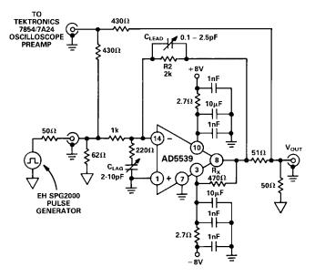
Figure 39. AD5539 Settling Time Test Circuit
