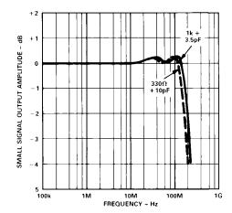
Figure 20. Response of the (Figure 17) Inverter Circuit with an  $R_{LAG}$  and a  $C_{LAG}$  Compensation Network **Employed**
