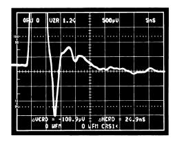
Figure 41. Error Signal from AD5539 Settling Time Test Circuit – Rising Edge. Vertical Scale: 5 ns/div.; Horizontal Scale: 500 µV/div
