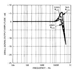
Figure 30. Response of the Gain of 3 Follower Circuit with  $C_{\rm LEAD}$  Connected to Pin 12
