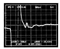
Figure 40. Error Signal from AD5539 Settling Time Test Circuit – Falling Edge. Vertical Scale: 5 ns/div.; Horizontal Scale: 500 µV/div
