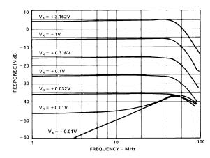
Figure 45. AC Response of the VCA at Different Gains  $V_V = 0.5 \ V \ RMS$
