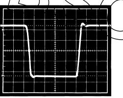
Figure 22. Large Signal Response of the (Figure 17) Inverter Circuit; Vertical Scale: 200 mV/div, Horizontal Scale: 5 ns/div
