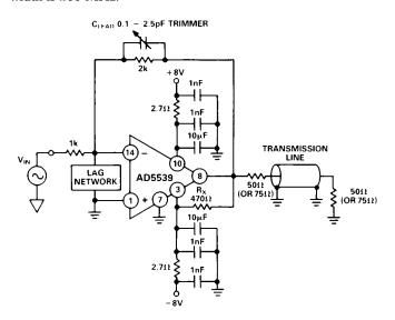
Figure 17. A General Purpose Inverter Circuit
