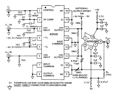
Figure 44. A Wide Bandwidth Voltage-Controlled Amplifier
