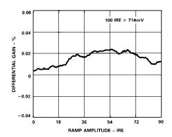
Figure 37. Differential Gain vs. Ramp Amplitude
