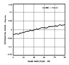
Figure 38. Differential Phase vs. Ramp Amplitude
