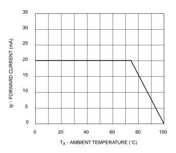
Fig. 5 Current Derating Curve
