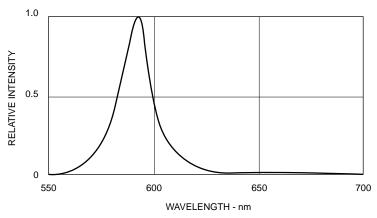
Fig. 3 Relative Intensity vs Peak Wavelength
