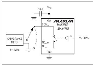
Figure 6. Channel Off/On-Capacitance
