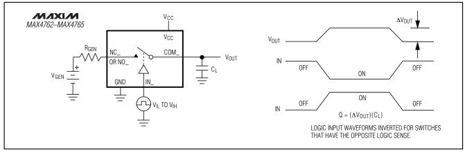
Figure 4. Charge Injection
