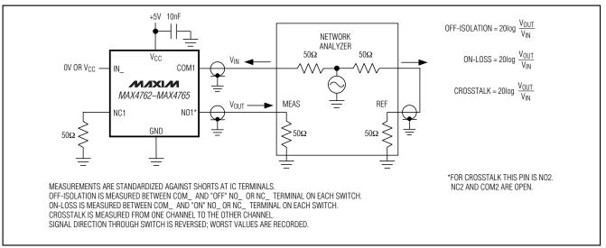
Figure 5. On-Loss, Off-Isolation, and Crosstalk
