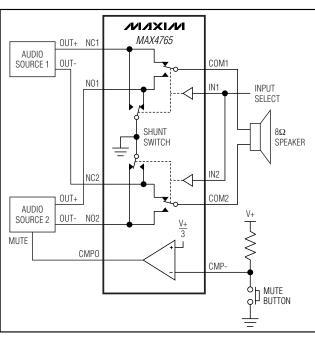
Figure 1. Typical Operating Circuit
