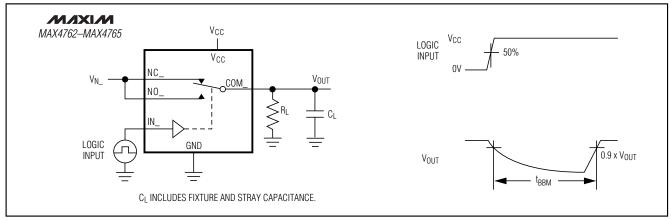
Figure 3. Break-Before-Make Interval
