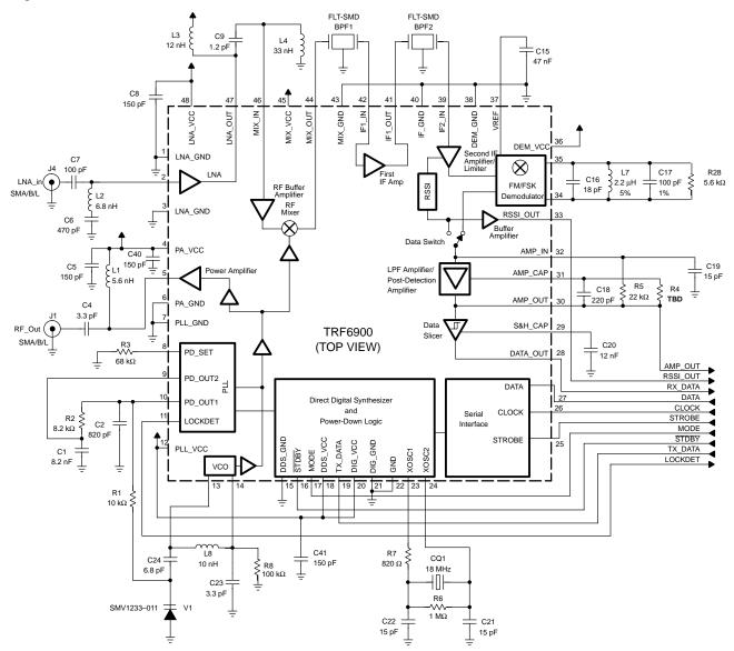
Figure 27. Typical Application Schematic for 868 to 870 MHz European ISM Band
