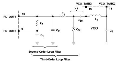
Figure 21. Basic Third-Order Loop Filter Structure
