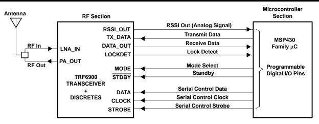
Figure 1. System Block Diagram for Interfacing to the MSP430 Microcontroller
