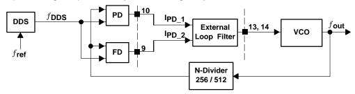
Figure 18. Basic PLL Structure
