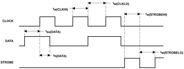
NOTE 2: CLOCK and DATA must both be low when STROBE is asserted (STROBE = 1).
