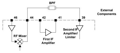
Figure 7. Bypassing the First IF Amplifier
