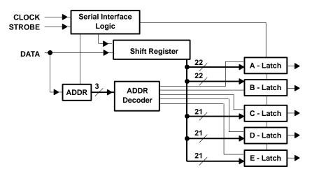
Figure 23. Serial Interface Block Diagram
