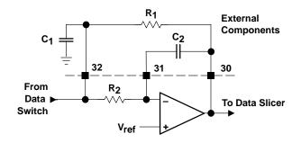
Figure 11. First-Order Low-Pass Filter Example
