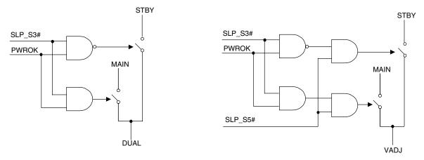
Figure 3. Control Logic for Dual Voltages and Memory Voltages
