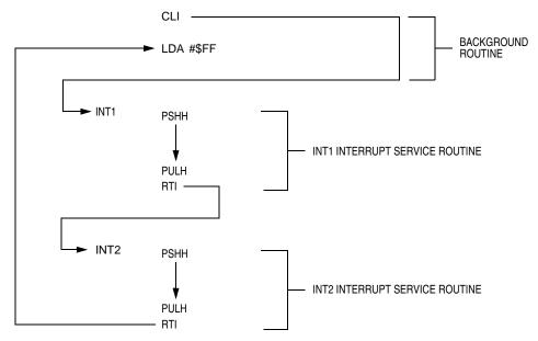
Figure 10-11. Interrupt Recognition Example
