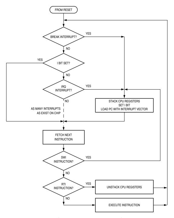
Figure 10-10. Interrupt Processing
