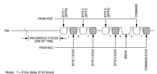
2 = Data return delay (2 bit times) 3 = Wait 1 bit time before sending next byte.
