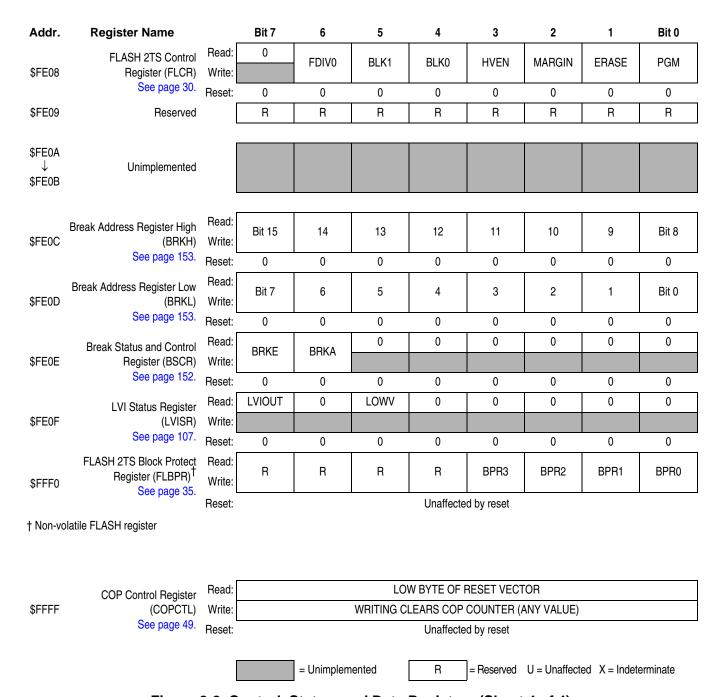
Figure 2-2. Control, Status, and Data Registers (Sheet 4 of 4)
