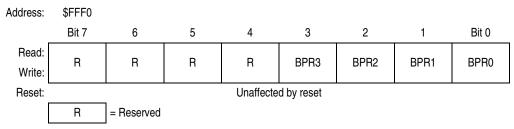
Figure 2-5. FLASH 2TS Block Protect Register (FLBPR)
