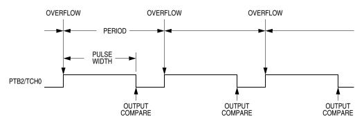
Figure 11-4. PWM Period and Pulse Width
