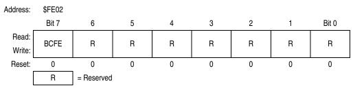
Figure 10-19. SIM Break Flag Control Register (SBFCR)
