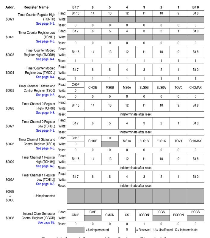
Figure 2-2. Control, Status, and Data Registers (Sheet 2 of 4)
