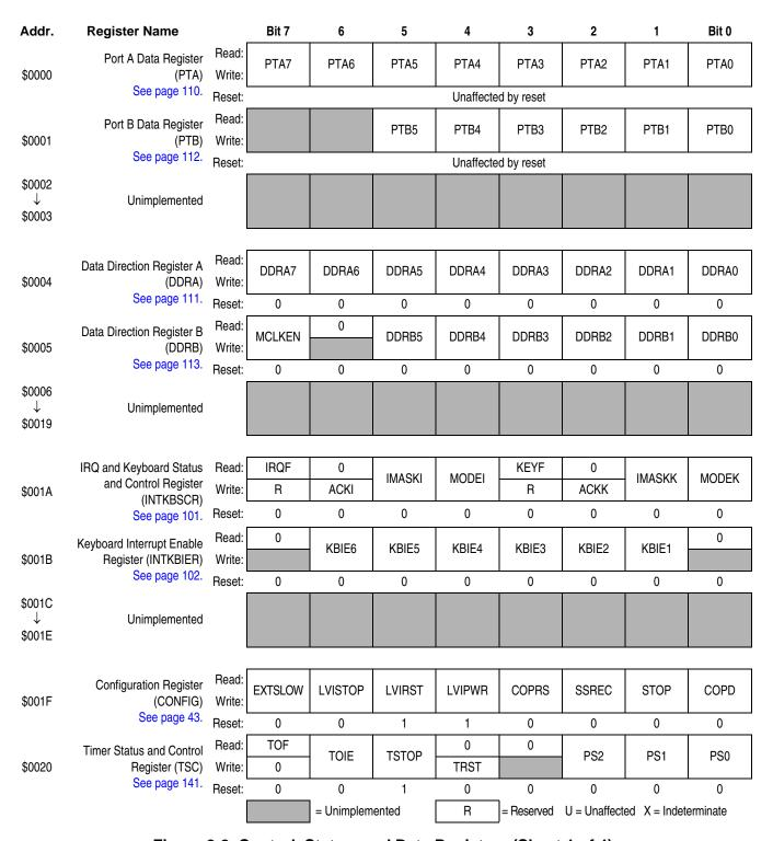
Figure 2-2. Control, Status, and Data Registers (Sheet 1 of 4)
