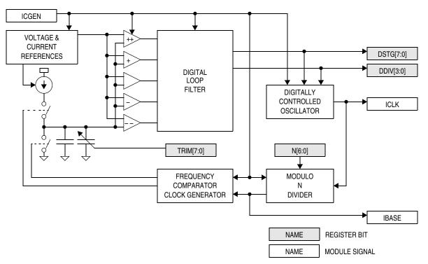
Figure 6-3. Internal Clock Generator Block Diagram
