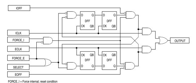
Figure 6-7. Synchronizing Clock Switcher Circuit Diagram
