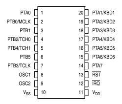
Figure 1-2. SSOP/SOIC Pin Assignments
