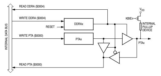
Figure 9-4. Port A I/O Circuit
