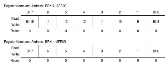
Figure 12-4. Break Address Registers (BRKH and BRKL)
