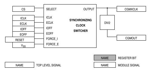
Figure 6-6. Clock Selection Circuit Block Diagram
