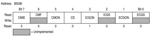
Figure 6-12. ICG Control Register (ICGCR)
