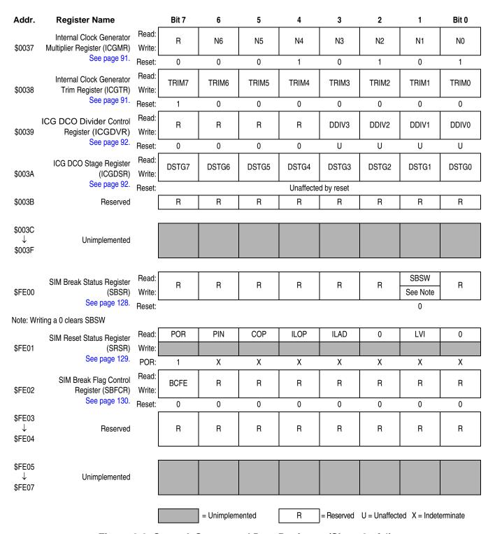
Figure 2-2. Control, Status, and Data Registers (Sheet 3 of 4)
