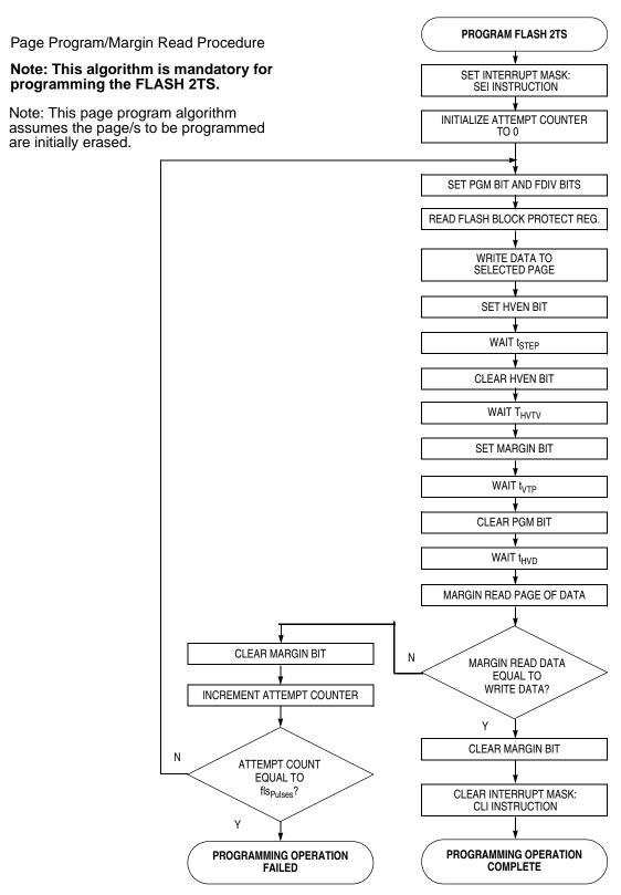
Figure 2-4. Smart Programming Algorithm Flowchart
