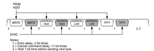
Figure 12-11. Write Transaction
