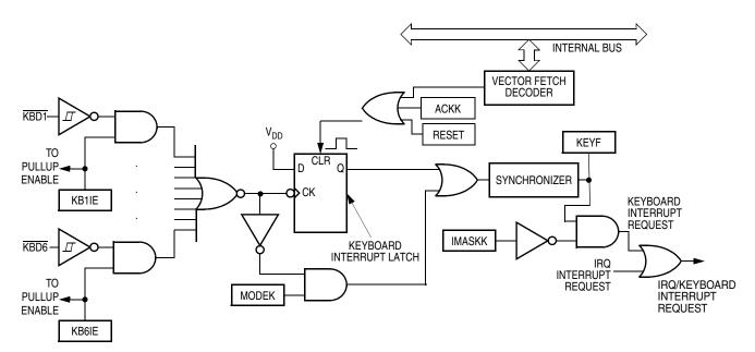
Figure 7-5. Keyboard Interrupt Block Diagram
