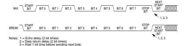
Figure 12-7. Sample Monitor Waveforms
