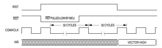
Figure 10-5. Internal Reset Timing
