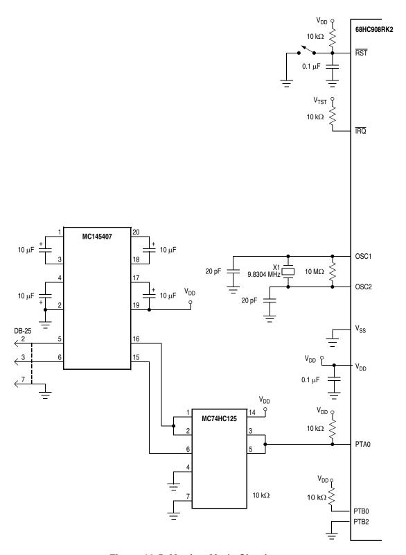
Figure 12-5. Monitor Mode Circuit
