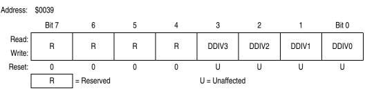
Figure 6-15. ICG DCO Divider Register (ICGDVR)
