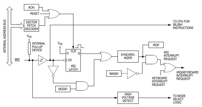
Figure 7-2. IRQ Block Diagram
