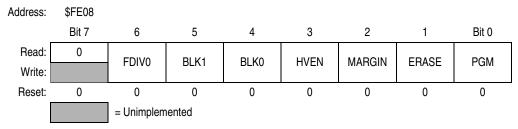
Figure 2-3. FLASH 2TS Control Register (FLCR)
