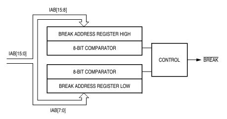
Figure 12-1. Break Module Block Diagram
