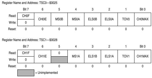
Figure 11-8. TIM Channel Status and Control Registers (TSC0 and TSC1)
