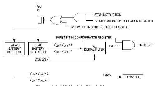
Figure 8-1. LVI Module Block Diagram
