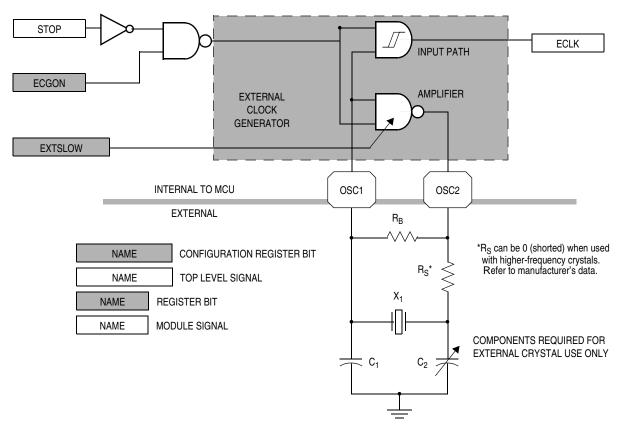
Figure 6-4. External Clock Generator Block Diagram
