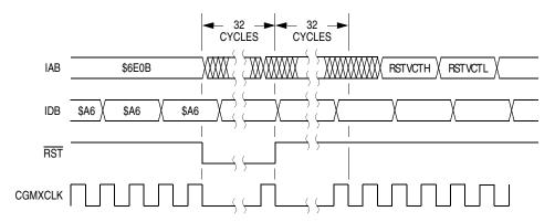
Figure 10-14. Wait Recovery from Internal Reset
