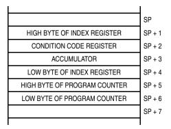
Figure 12-12. Stack Pointer at Monitor Mode Entry
