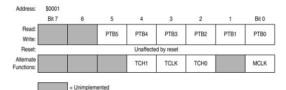
Figure 9-5. Port B Data Register (PTB)
