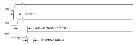
Note: Any delay between rising  $\overline{IRQ}$  and rising  $V_{DD}$  will guarantee that the MCU bus is driven by the external clock.
