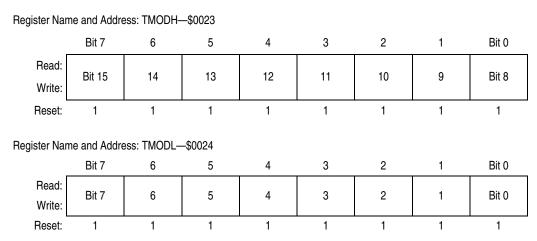
Figure 11-7. TIM Counter Modulo Registers (TMODH and TMODL)
