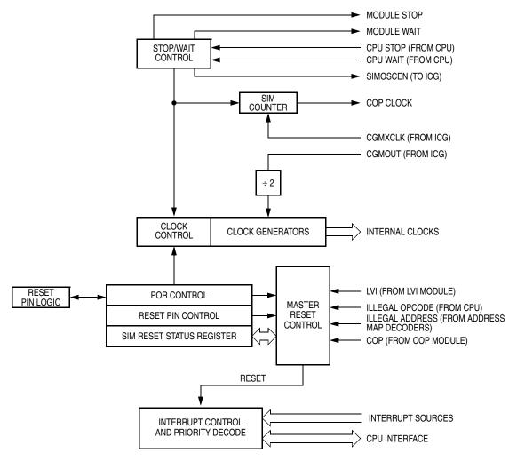
Figure 10-2. SIM Block Diagram
