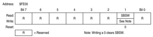
Figure 10-17. SIM Break Status Register (SBSR)
