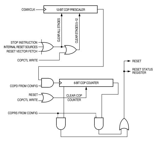
Figure 4-1. COP Block Diagram
