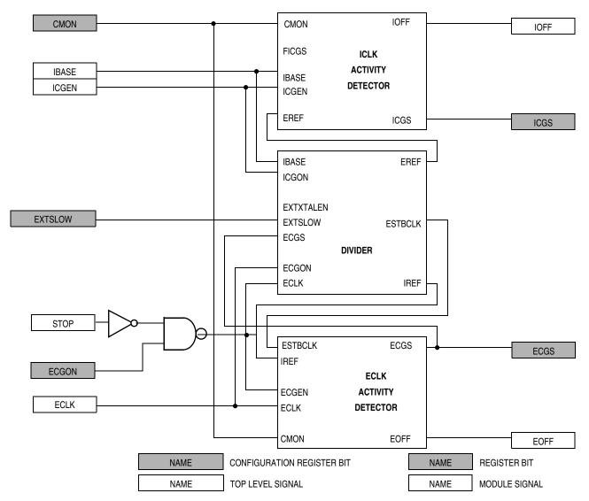
Figure 6-5. Clock Monitor Block Diagram
