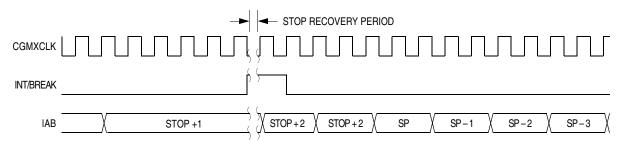
Figure 10-16. Stop Mode Recovery from Interrupt or Break
