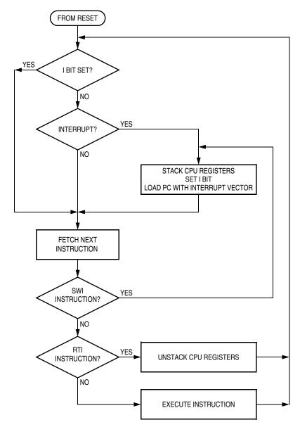
Figure 7-4. IRQ Interrupt Flowchart
