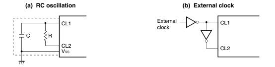
Caution When using the system clock oscillator, wire as follows in the area enclosed by the broken lines in Figure 8-3 to avoid an adverse effect from wiring capacitance.
