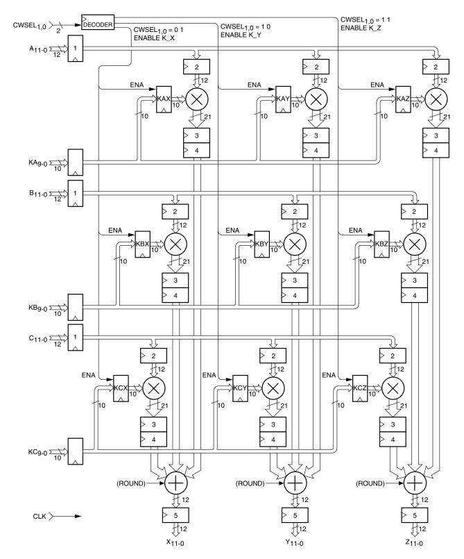
The TMC2272A is a nine-multiplier array with the internal bus structure and summing adders needed to implement a 3 x 3 matrix multiplier (triple dot product). With a 50MHz guaranteed maximum clock rate, this device offers video and imaging system designers a single-chip solution to numerous common image and signal-processing problems.
