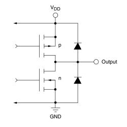
Figure 5. Equivalent Digital Input Circuit
