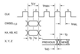
Figure 2. Input/Output Timing
