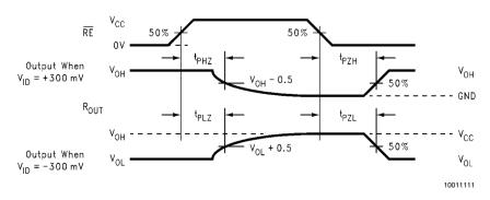
FIGURE 9. Receiver TRI-STATE Delay Waveforms
