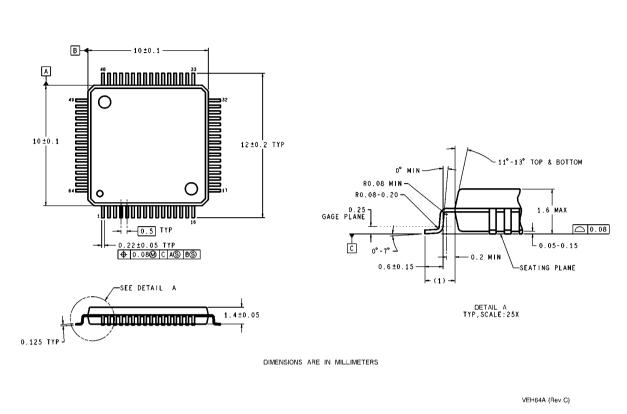
64-Lead Molded TQFP Package Order Number DS92LV090ATVEH NS Package Number VEH064DB
