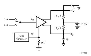
FIGURE 4. Driver TRI-STATE Delay Test Circuit
