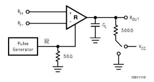
FIGURE 8. Receiver TRI-STATE Delay Test Circuit
