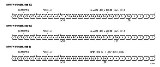
Figure 2. Command and Data Input Format
