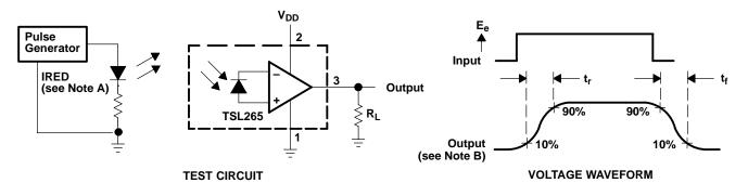
NOTES: A. The input irradiance is supplied by a pulsed GaAlAs infrared-emitting diode with the following characteristics:  $\lambda_p$  = 880 nm,  $t_r < 1 \ \mu$ s.
