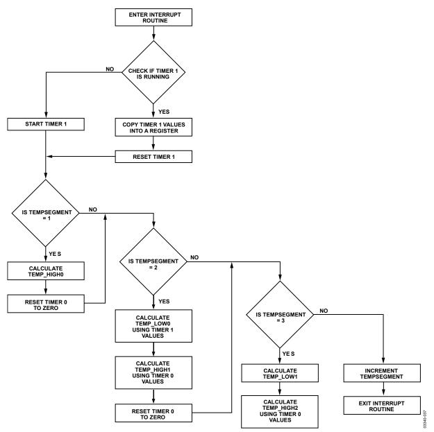
Figure 36. ADuC812 Interrupt Routine Flowchart
