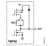
Figure 23. TMP05 One Shot Mode OUT Pin Configuration
