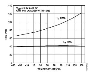
Figure 8.  $T_H$  and  $T_L$  Times vs. Temperature
