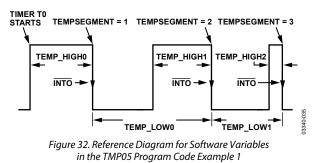
Figure 32 is a diagram of the input waveform into the ADuC812 from the TMP05 daisy chain. It illustrates how the code's variables are assigned and it should be referenced when reading the TMP05 Program Code Example 1. Application notes showing the TMP05 working with other types of microcontrollers are available from Analog Devices at www.analog.com.
