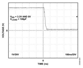
Figure 10. TMP05 Output Fall Time at 25°C
