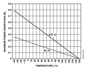
Figure 4. Maximum Power Dissipation vs. Ambient Temperature
