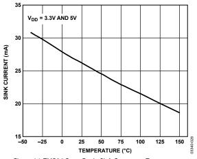
Figure 14. TMP06 Open Drain Sink Current vs. Temperature
