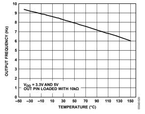
Figure 6. PWM Output Frequency vs. Temperature
