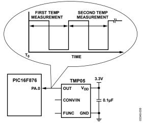
Figure 37. Typical Continuously Converting Application Circuit
