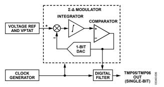
Figure 20. First-Order  $\Sigma$ - $\Delta$  Modulator
