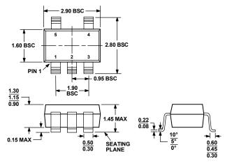
COMPLIANT TO JEDEC STANDARDS MO-178-AA Figure 39. 5-Lead Small Outline Transistor Package [SOT-23] (RJ-5)
