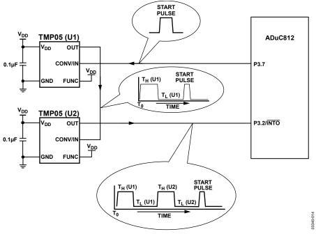
Figure 33. Typical Daisy-Chain Application Circuit
