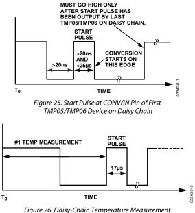
and Start Pulse Output from First TMP05/TMP06
