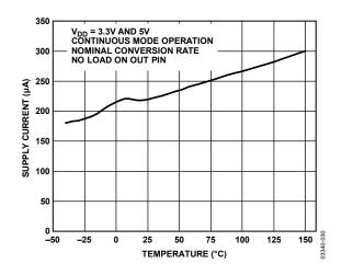
Figure 16. Supply Current vs. Temperature
