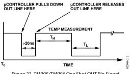
Figure 22. TMP05/TMP06 One Shot OUT Pin Signal
