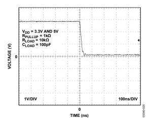
Figure 11. TMP06 Output Fall Time at 25°C
