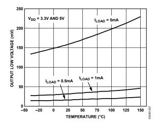
Figure 13. TMP06 Output Low Voltage vs. Temperature
