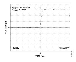
Figure 9. TMP05 Output Rise Time at 25°C
