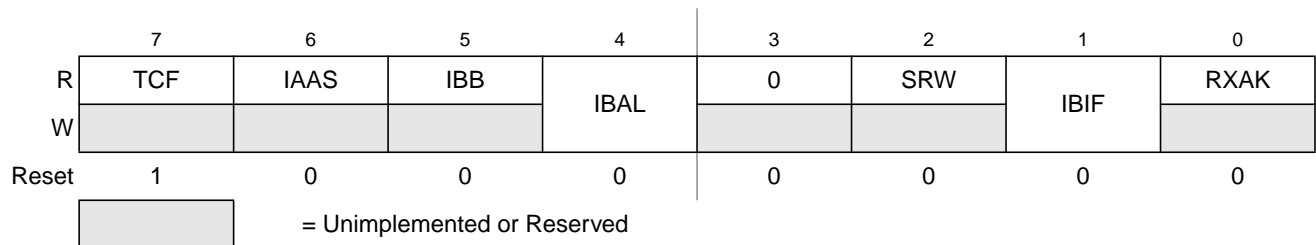
Figure 11-6. IIC Bus Status Register (IBSR)
