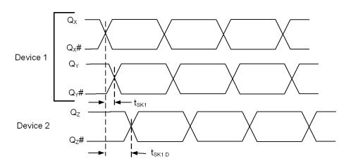
Figure 7. RMS Phase Jitter
