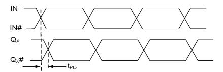
Figure 5. Output Duty Cycle
