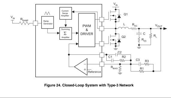
FAN5069 has a high gain error amplifier around which the loop is closed. Figure 24 shows a Type-3 compensation network. For Type-2 compensation, R3 and C3 are not used. Since the FAN5069 architecture employs summing current mode, Type-2 compensation can be used for most applications. For further information about Type-2 compensation networks, refer to:
