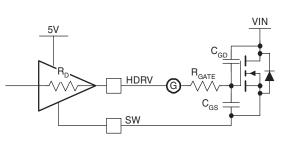
Figure 23. Drive Equivalent Circuit
