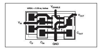
Figure 3. Suggested PCB Design for Minimum Ripple
