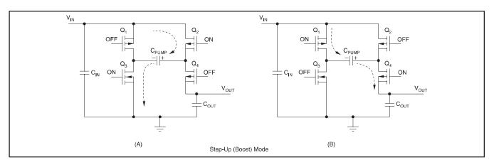
Figure 1. Simplified Schematic of the SN0304078 Operating in the Step-Up or Boost Mode
