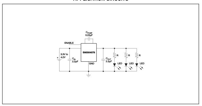
Figure 4. SN0304078 Circuit for Driving LEDs
