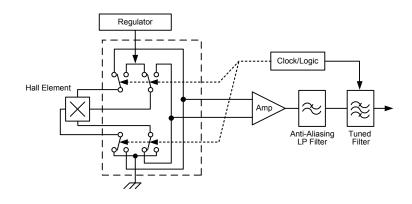
Figure 4. Chopper stabilization technique
