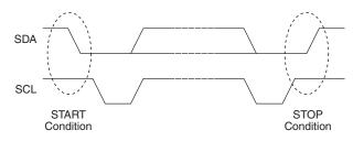
This protocol uniquely defines START and STOP conditions. A START condition is defined as a HIGH to LOW transition of the SDA signal while SCL is HIGH. A STOP condition is defined as a LOW to HIGH transition of the SDA signal while SCL is HIGH. These are shown in Figure 2.
