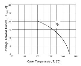
Figure 6. Forward Current Derating Curve
