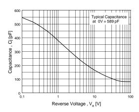
Figure 3. Typical Junction Capacitance
