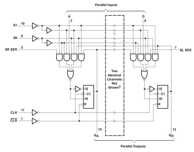
$\dagger$  I/O ports not shown: QB (14) and QC (13) Pin numbers shown are for the D, J, and N packages.
