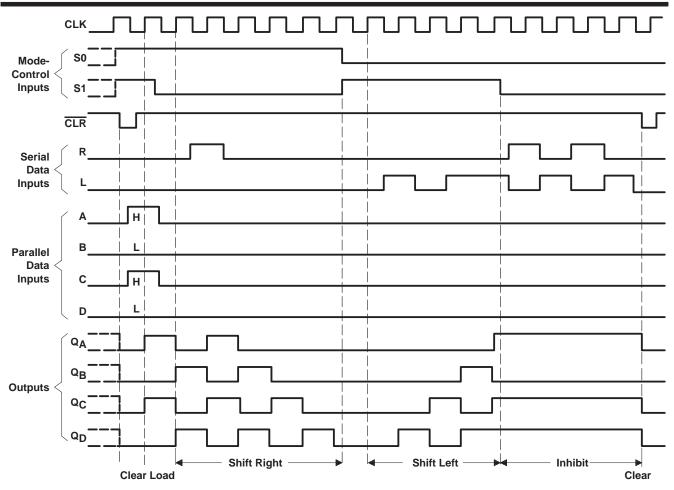
Figure 1. Typical Clear, Load, Right-Shift, and Clear Sequences
