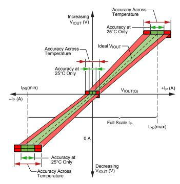
Figure 5: Output Voltage versus Sensed Current
