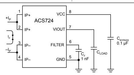
The ACS724 outputs an analog signal, V<sub>IOUT</sub>, that changes proportionally with the bidirectional AC or DC primary sensed current, I<sub>P</sub>, within the specified measurement range. The FILTER pin can be used to decrease the bandwidth in order to optimize the noise performance.
