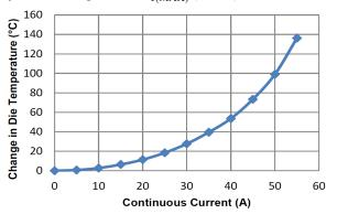
Figure 2: Self Heating in the LC Package
