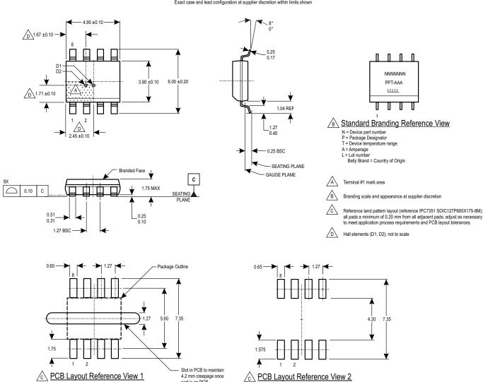
Figure 7: Package LC, 8-pin SOICN
