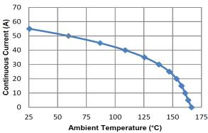
Figure 3: Maximum Continuous Current at a Given T<sub>△</sub>
