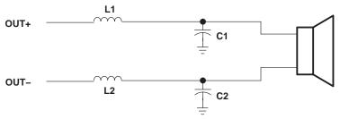
Figure 1. Class-D Output Filter
