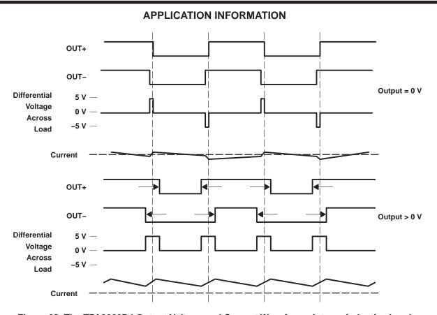
Figure 28. The TPA2000D4 Output Voltage and Current Waveforms Into an Inductive Load
