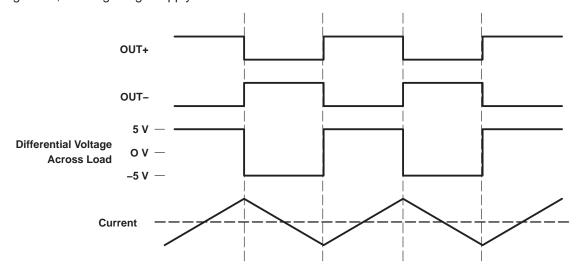
Figure 27. Traditional Class-D Modulation Scheme's Output Voltage and Current Waveforms Into an Inductive Load With No Input
