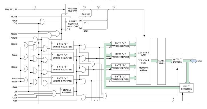
**NOTE:** Functional Block Diagrams illustrate simplified device operation. See Truth Table, Pin Descriptions and timing diagrams for detailed information.
