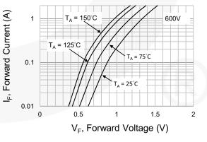
Figure 6. Typical Forward Characteristics
