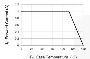
**Figure 1. Forward Current Derating Curve**
