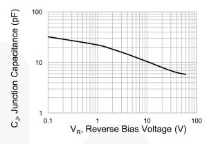
Figure 2. Typical Junction Capacitance
