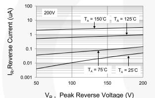
Figure 3. Typical Reverse Characteristics
