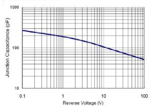
**Figure 5. Typical Junction Capacitance**
