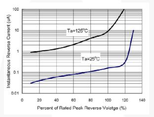
Figure 3. Typical Reverse Characteristics per Leg
