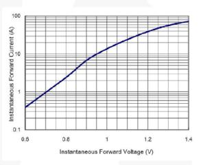
Figure 4. Typical Forward Characteristics per Leg
