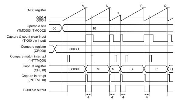
This is an application example where the width set to CR000 (4 clocks in this example) is to be output from the TO00 pin when the count value has been captured & cleared.
