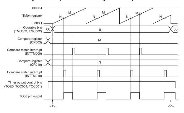
Figure 6-39. Example of Software Processing in Free-Running Timer Mode
