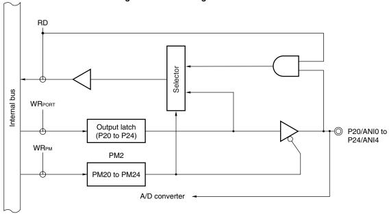
Figure 4-9. Block Diagram of P20 to P24
