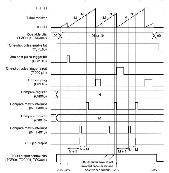
Figure 6-45. Example of Software Processing for One-Shot Pulse Output Operation (1/2)
