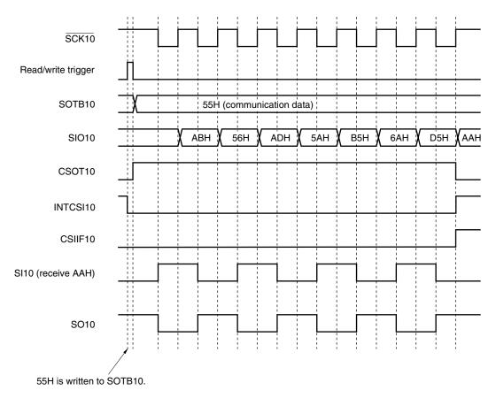
Figure 15-5. Timing in 3-Wire Serial I/O Mode (2/2)
