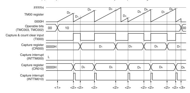
Figure 6-52. Example of Software Processing for Pulse Width Measurement (2/2)
