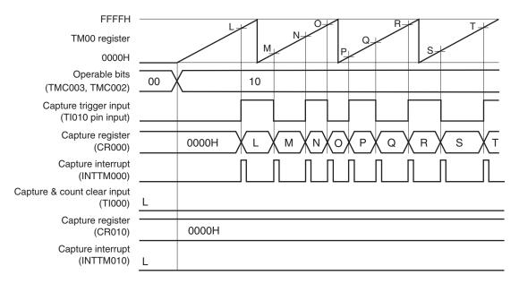
This is a timing example where an edge is not input to the Tl000 pin, in an application where the count value is captured to CR000 when the rising or falling edge of the Tl010 pin is detected.
