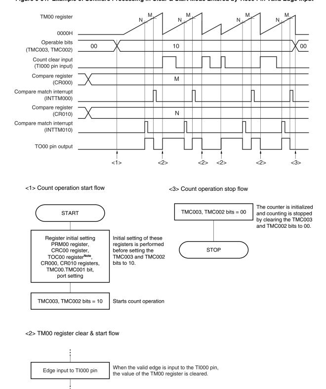
Figure 6-31. Example of Software Processing in Clear & Start Mode Entered by Tl000 Pin Valid Edge Input
