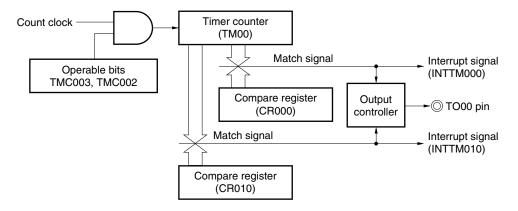
Figure 6-33. Timing Example of Free-Running Timer Mode (CR000: Compare Register, CR010: Compare Register)
