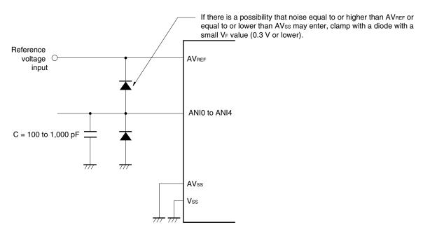
Figure 12-20. Analog Input Pin Connection
