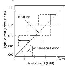
Figure 12-18. Integral Linearity Error
