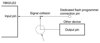
In the flash memory programming mode, the signal output by the device collides with the signal sent from the dedicated flash programmer. Therefore, isolate the signal of the other device.
