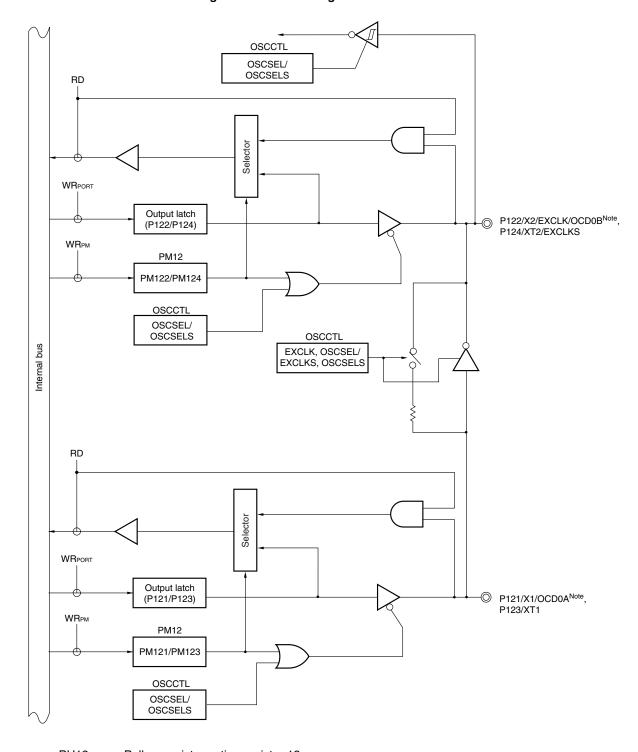
Figure 4-14. Block Diagram of P121 to P124
