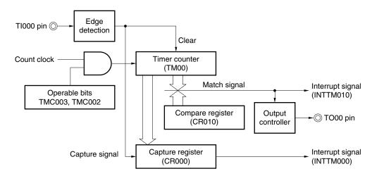
Figure 6-27. Timing Example of Clear & Start Mode Entered by Tl000 Pin Valid Edge Input (CR000: Capture Register, CR010: Compare Register) (1/2)
