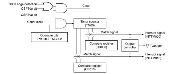
Figure 6-43. Block Diagram of One-Shot Pulse Output Operation
