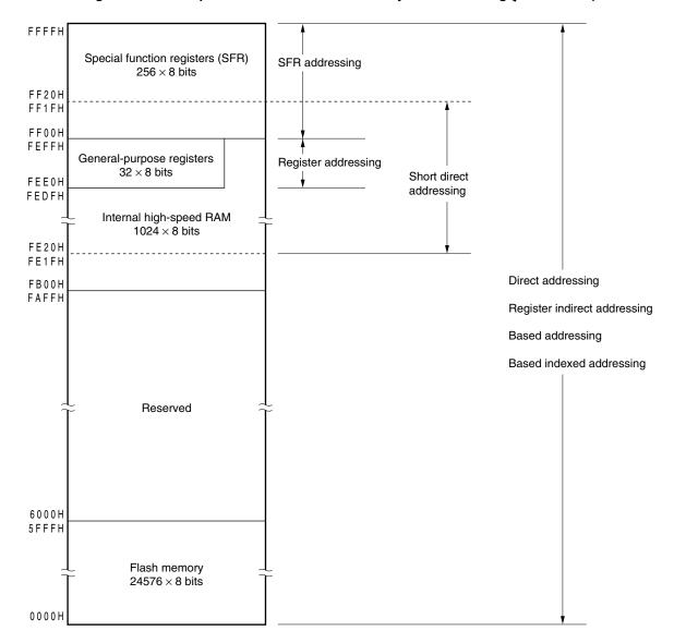
Figure 3-6. Correspondence Between Data Memory and Addressing (µPD78F0362)
