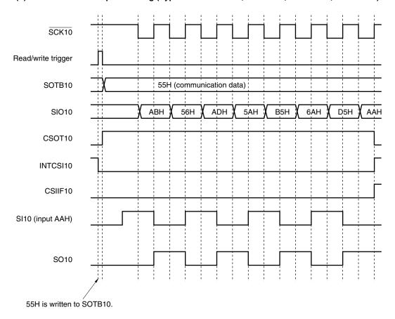
Figure 15-6. Timing of Clock/Data Phase
