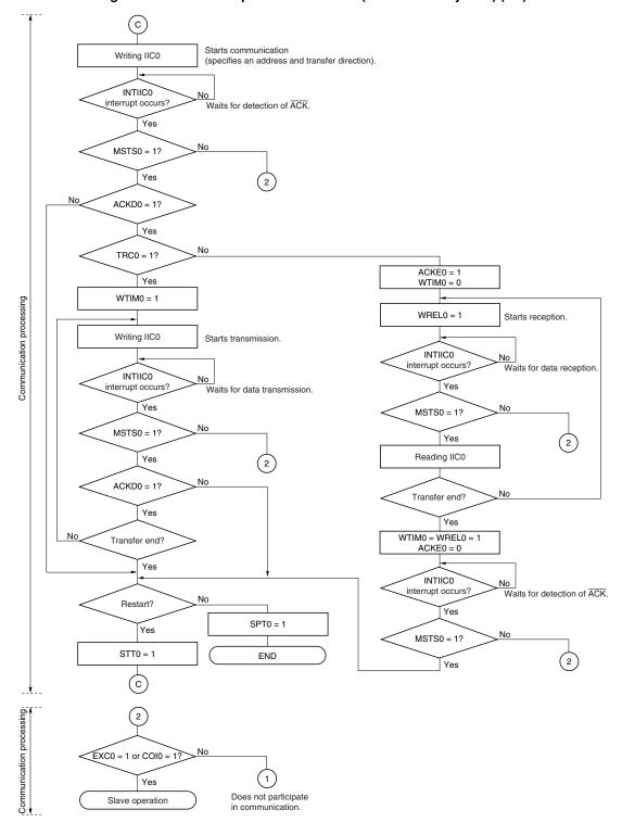
Figure 16-24. Master Operation Flowchart (Multi-Master System) (3/3)
