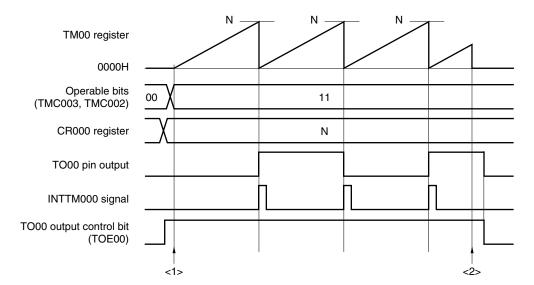
Figure 6-18. Example of Software Processing for Square Wave Output Function
