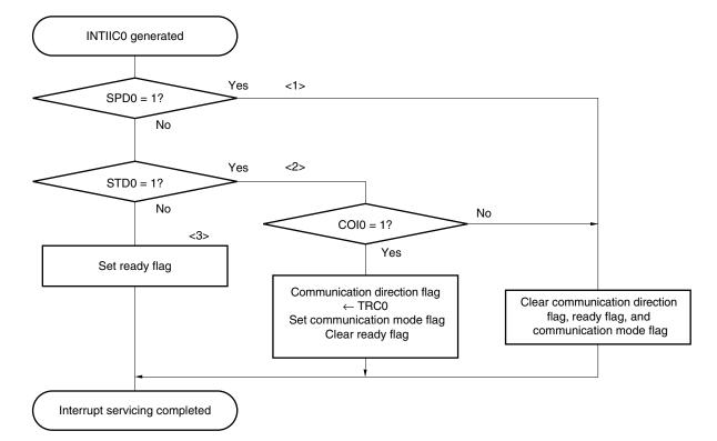
Figure 16-26. Slave Operation Flowchart (2)
