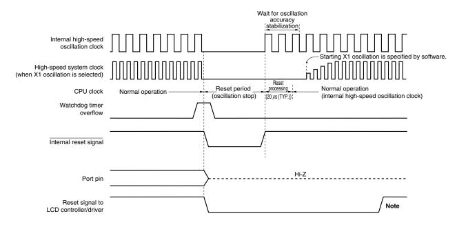
Figure 20-3. Timing of Reset Due to Watchdog Timer Overflow
