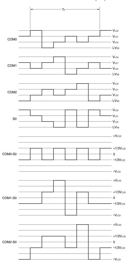
Figure 17-24. Three-Time-Slice LCD Drive Waveform Examples (1/3 Bias Method)
