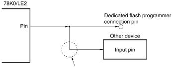
If the signal output by the 78K0/LE2 in the flash memory programming mode affects the other device, isolate the signal of the other device.
