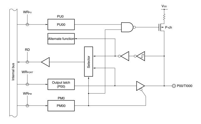
PU0: Pull-up resistor option register 0
