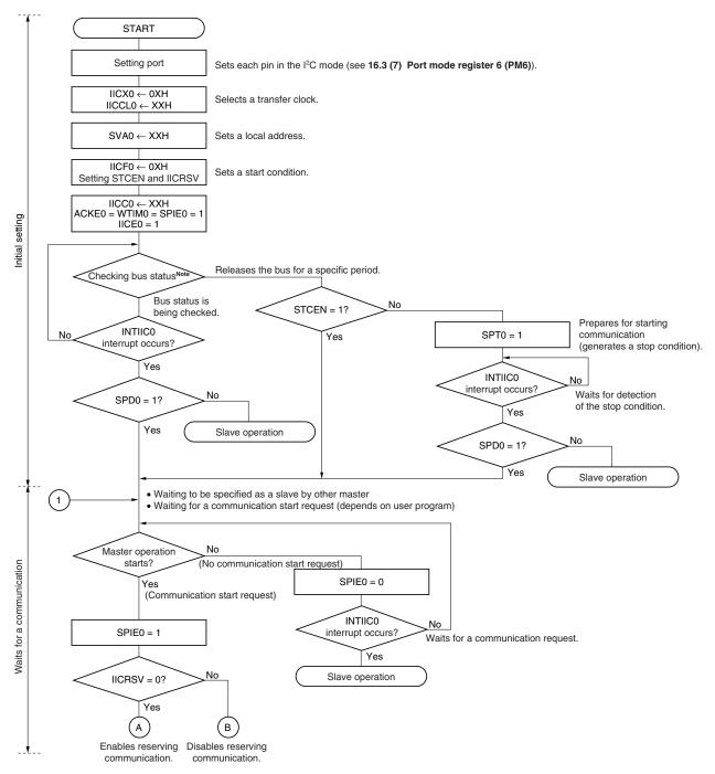
Note Confirm that the bus is released (CLD0 bit = 1, DAD0 bit = 1) for a specific period (for example, for a period of one frame). If the SDA0 pin is constantly at low level, decide whether to release the I<sup>2</sup>C bus (SCL0 and SDA0 pins = high level) in conformance with the specifications of the product that is communicating.
