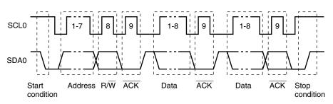
Figure 16-12. I<sup>2</sup>C Bus Serial Data Transfer Timing
