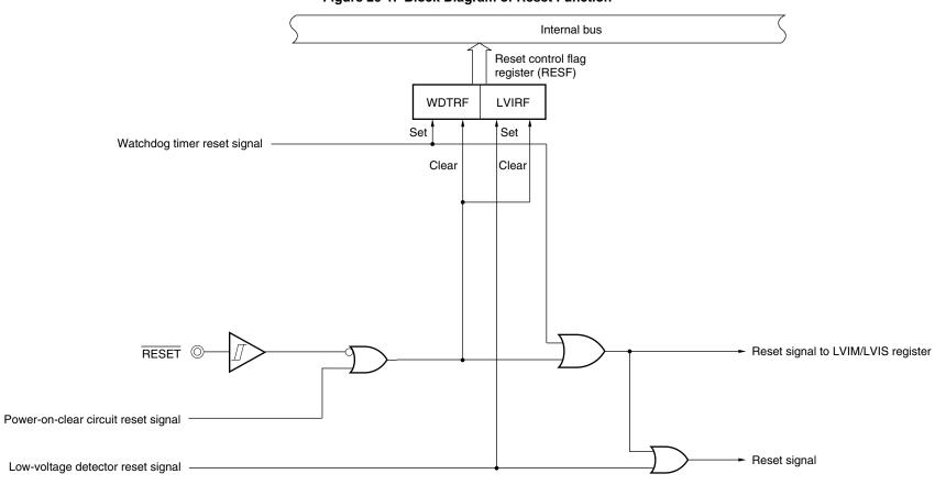
Figure 20-1. Block Diagram of Reset Function
