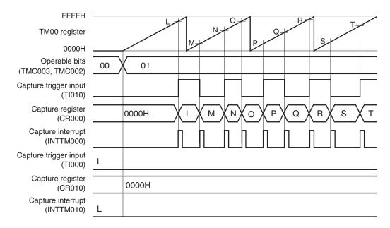
This is an application example where both the edges of the Tl010 pin are detected and the count value is captured to CR000 in the free-running timer mode.
