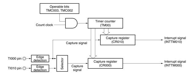
Figure 6-47. Block Diagram of Pulse Width Measurement (Clear & Start Mode Entered by Tl000 Pin Valid Edge Input)
