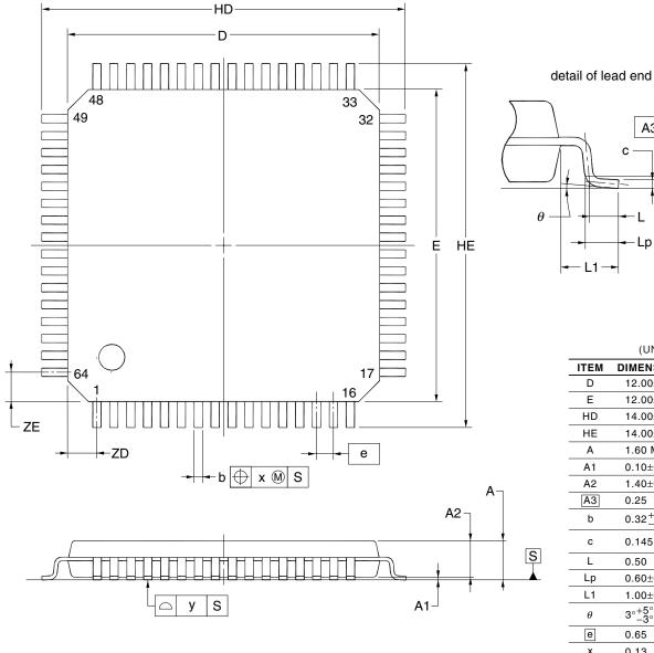
NOTE Each lead centerline is located within 0.13 mm of its true position at maximum material condition.
