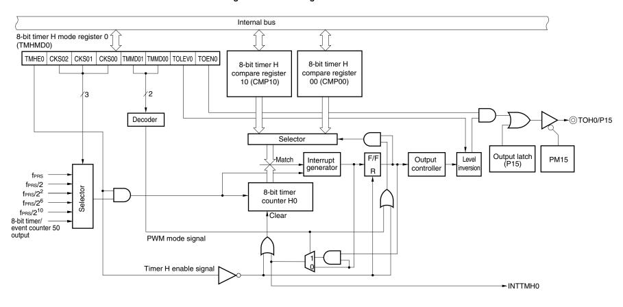
Figure 8-1. Block Diagram of 8-Bit Timer H0
