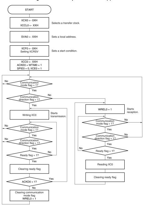
Figure 16-25. Slave Operation Flowchart (1)
