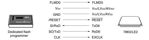
If FlashPro4 is used as the dedicated flash programmer, FlashPro4 generates the following signal for the 78K0/LE2. For details, refer to the FlashPro4 manual.
