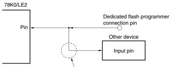
If the signal output by the dedicated flash programmer in the flash memory programming mode affects the other device, isolate the signal of the other device.
