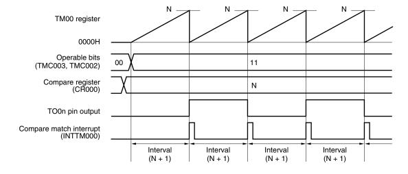
Figure 6-17. Example of Register Settings for Square Wave Output Operation
