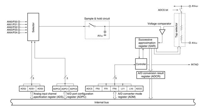
Figure 12-1. Block Diagram of A/D Converter
