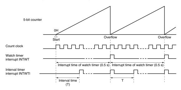
Figure 9-3. Operation Timing of Watch Timer/Interval Timer
