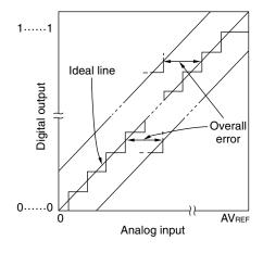
Figure 12-15. Quantization Error
