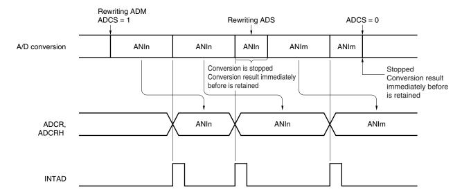
Figure 12-13. A/D Conversion Operation
