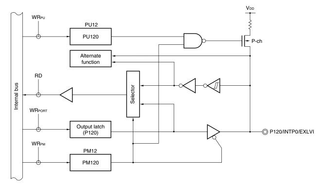
Figure 4-13. Block Diagram of P120
