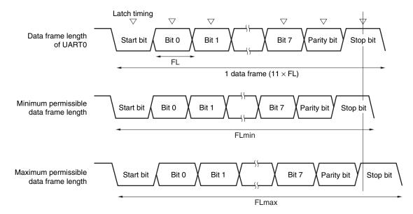
Figure 13-12. Permissible Baud Rate Range During Reception
