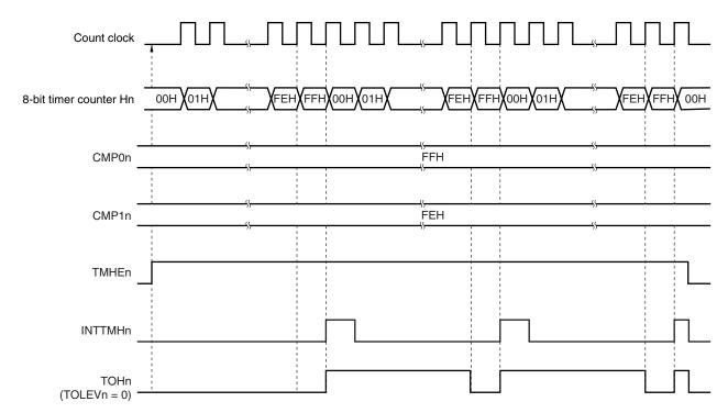
Figure 8-12. Operation Timing in PWM Output Mode (3/4)
