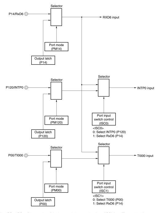
Figure 14-3. Port Configuration for LIN Reception Operation
