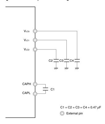
Figure 17-30. Example of Connecting Pins for LCD Driver
