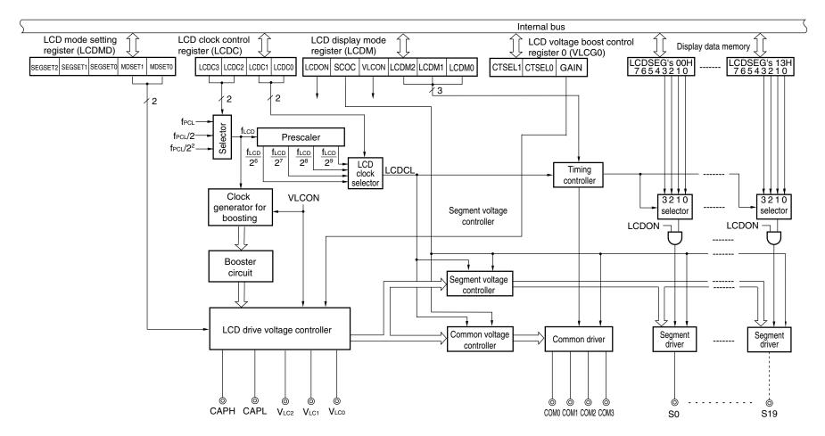
Remark fpcl: The clock generated by the clock output controller
