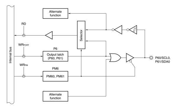
Figure 4-12 Block Diagram of P60 and P61
