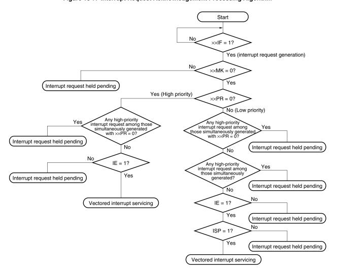
Figure 18-7. Interrupt Request Acknowledgement Processing Algorithm
