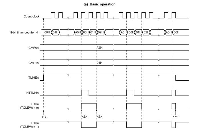
Figure 8-12. Operation Timing in PWM Output Mode (1/4)
