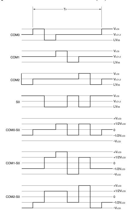
Figure 17-23. Three-Time-Slice LCD Drive Waveform Examples (1/2 Bias Method)
