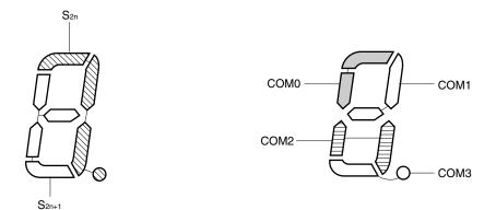
Figure 17-25. Four-Time-Slice LCD Display Pattern and Electrode Connections
