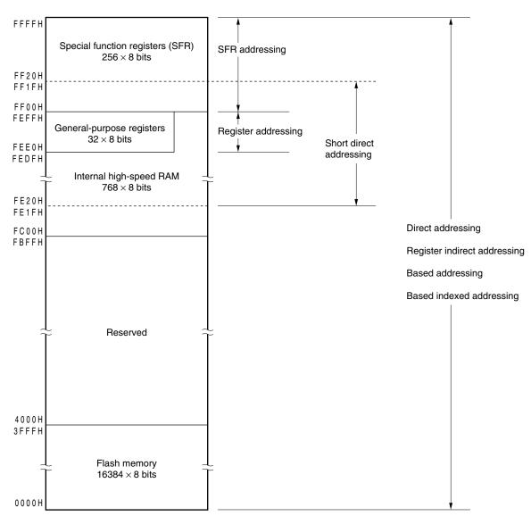
Figure 3-5. Correspondence Between Data Memory and Addressing (µPD78F0361)
