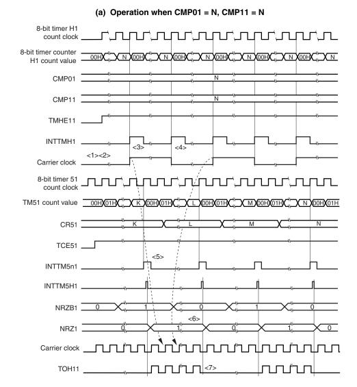
Figure 8-15. Carrier Generator Mode Operation Timing (1/3)
