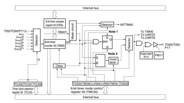
Figure 7-1. Block Diagram of 8-Bit Timer/Event Counter 50
