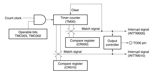
Figure 6-40. Block Diagram of PPG Output Operation
