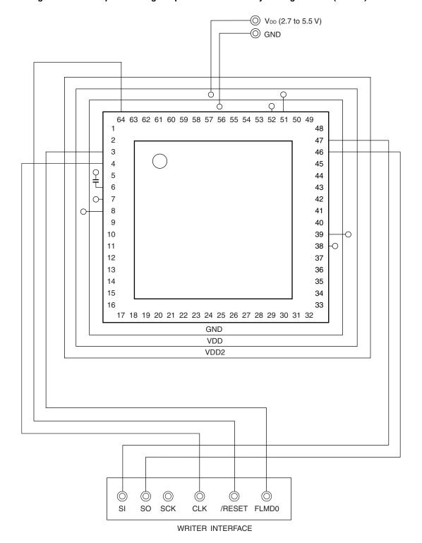
Figure 24-3. Example of Wiring Adapter for Flash Memory Writing in UART (UART6) Mode
