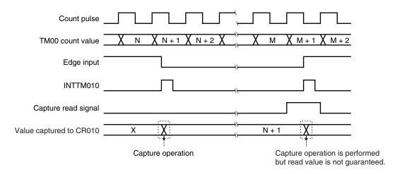
Figure 6-56. Timing of Holding Data by Capture Register
