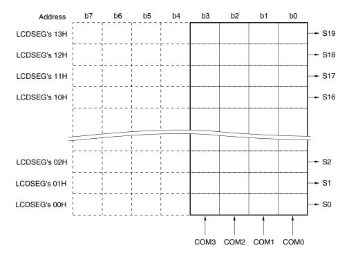
Caution No memory is allocated to the higher 4 bits of the LCD display data memory. Be sure to set there bits to 0.
