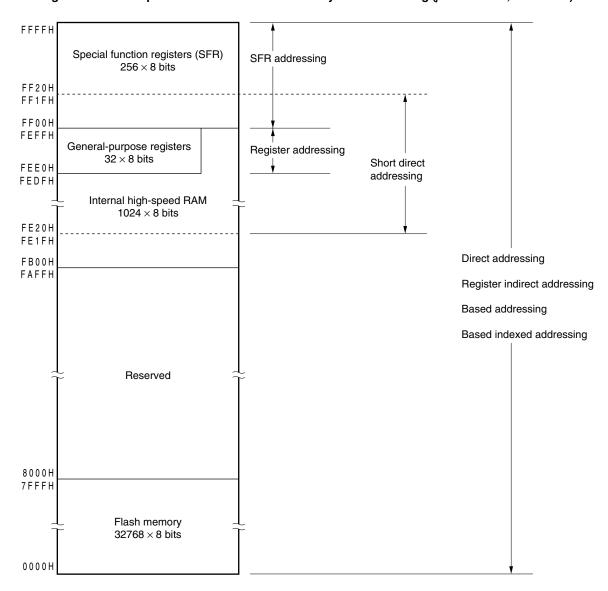
Figure 3-7. Correspondence Between Data Memory and Addressing (µPD78F0363, 78F0363D)
