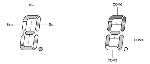
Figure 17-21. Three-Time-Slice LCD Display Pattern and Electrode Connections
