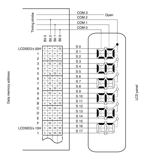
Figure 17-22. Example of Connecting Three-Time-Slice LCD Panel
