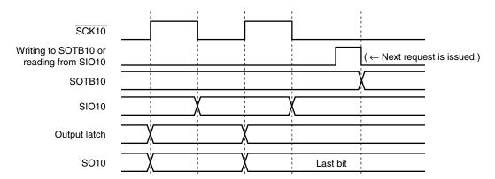
Figure 15-8. Output Value of SO10 Pin (Last Bit) (2/2)
