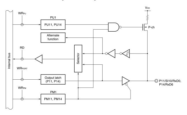
Figure 4-5. Block Diagram of P11 and P14
