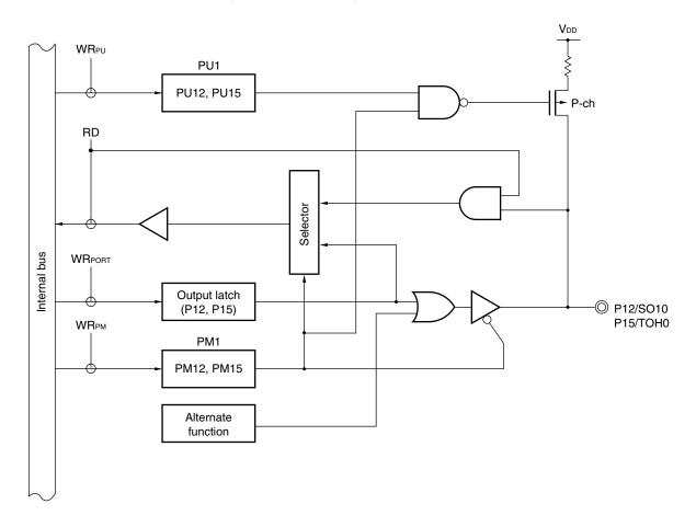
Figure 4-6. Block Diagram of P12 and P15
