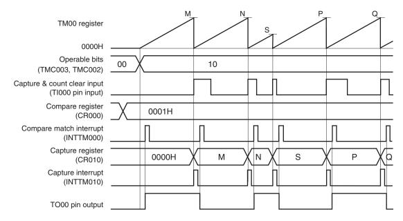
This is an application example where the output level of the TO00 pin is inverted when the count value has been captured & cleared.
