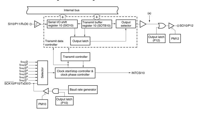
Figure 15-1. Block Diagram of Serial Interface CSI10
