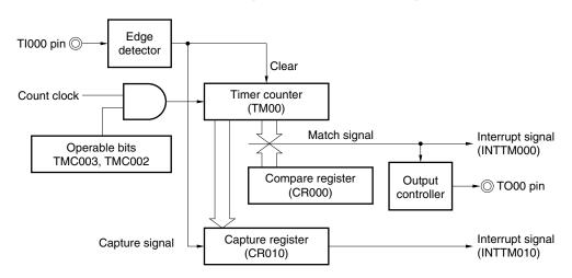
Figure 6-25. Timing Example of Clear & Start Mode Entered by Tl000 Pin Valid Edge Input (CR000: Compare Register, CR010: Capture Register) (1/2)
