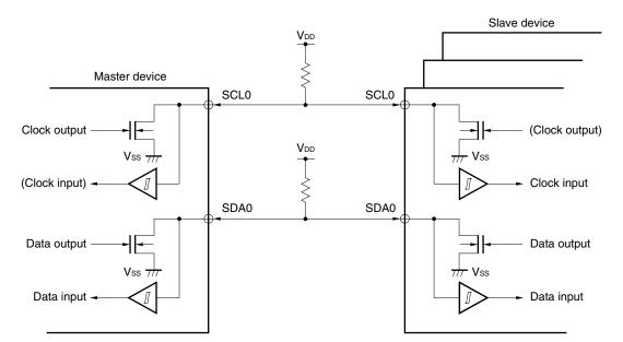
Figure 16-11. Pin Configuration Diagram
