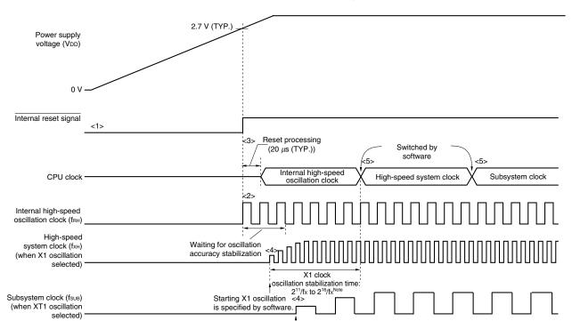
Figure 5-13. Clock Generator Operation When Power Supply Voltage Is Turned On (When 2.7 V/1.59 V POC Mode Is Set (Option Byte: POCMODE = 1))
