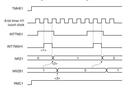
Figure 8-13. Transfer Timing
