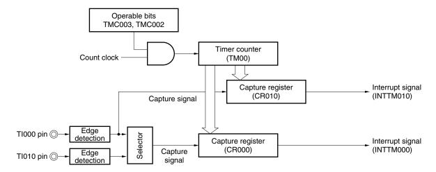
**Remark** If both CR000 and CR010 are used as capture registers in the free-running timer mode, the output level of the TO00 pin is not inverted.
