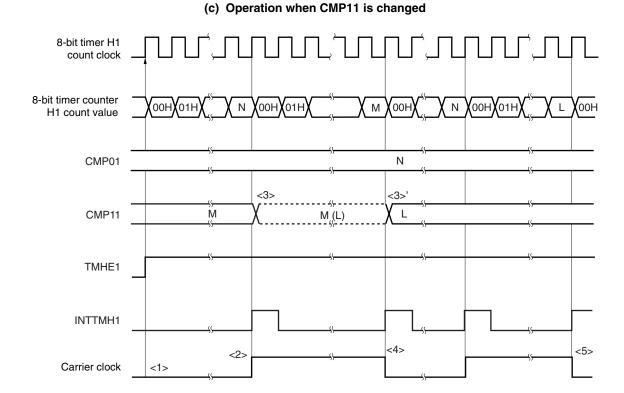
Figure 8-15. Carrier Generator Mode Operation Timing (3/3)
