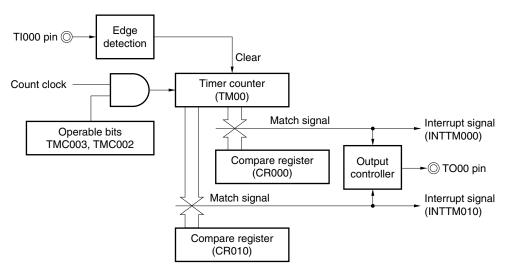
Figure 6-23. Timing Example of Clear & Start Mode Entered by Tl000 Pin Valid Edge Input (CR000: Compare Register, CR010: Compare Register)
