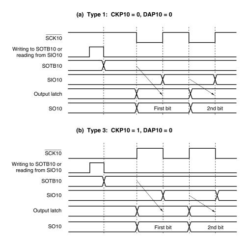
Figure 15-7. Output Operation of First Bit (1/2)
