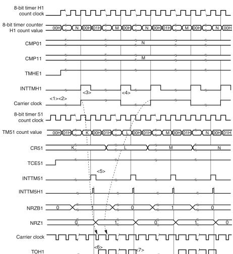
Figure 8-15. Carrier Generator Mode Operation Timing (2/3)
