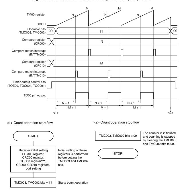
Figure 6-42. Example of Software Processing for PPG Output Operation
