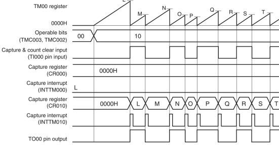
This is an application example where the count value is captured to CR010, TM00 is cleared, and the TO00 pin output is inverted when the rising or falling edge of the Tl000 pin is detected.
