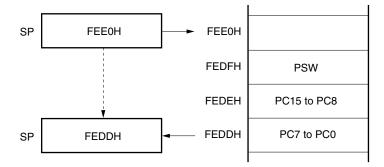
Figure 3-12. Data to Be Restored from Stack Memory
