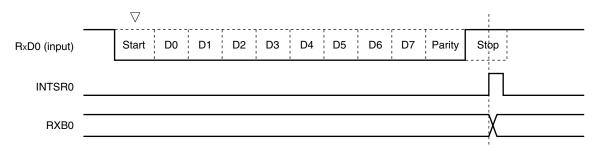
Figure 13-9. Reception Completion Interrupt Request Timing
