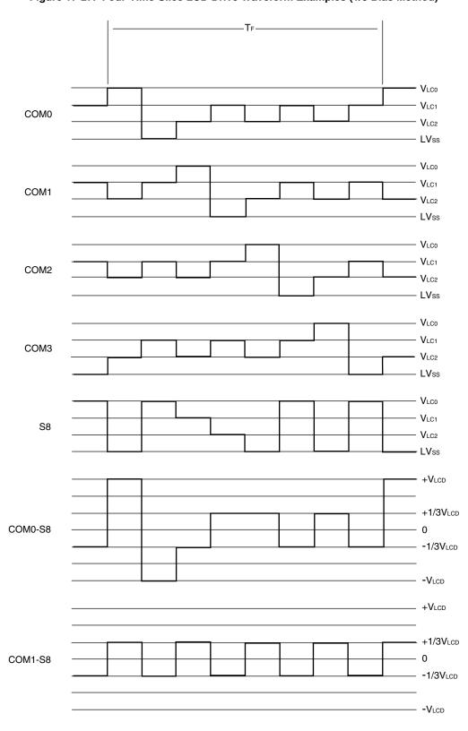
Figure 17-27. Four-Time-Slice LCD Drive Waveform Examples (1/3 Bias Method)
