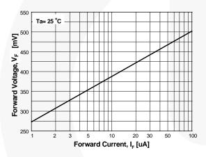
Figure 3. Forward Voltage vs. Forward Current  $\mbox{\sc V}_{\mbox{\sc F}}$  - 1 to 100  $\mbox{\sc {\sc H}}\mbox{\sc A}$
