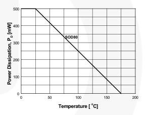
Figure 10. Power Derating Curve
