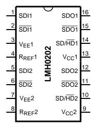
Figure 1. 16-Pin TSSOP See PW Package
