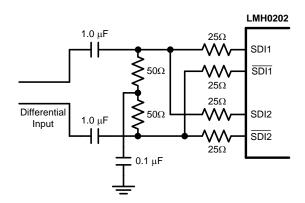
Figure 3. Single Differential Input for DVB-ASI
