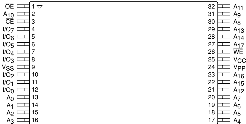
TSOP Package (Reverse Pinout) (TR, HR)
