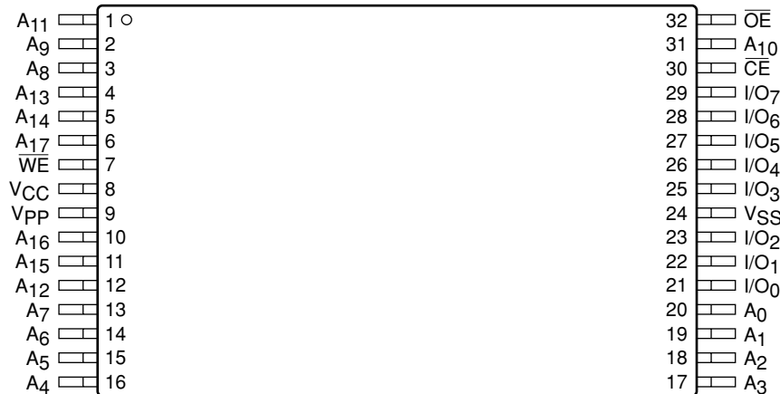
TSOP Package (Standard Pinout) (T, H)
