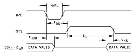
LOW PULSE FOR R/C - OUTPUTS ENABLED
