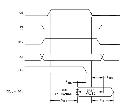
FIGURE 6. Read cycle timing.
