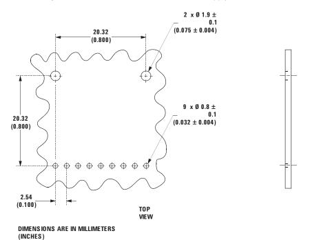
Figure 4. Recommended Board Layout Hole Pattern.
