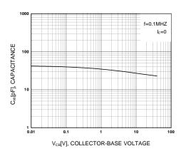
Figure 4. Collector Output Capacitance
