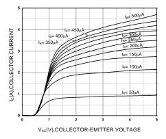
Figure 1. Static Characteristic
