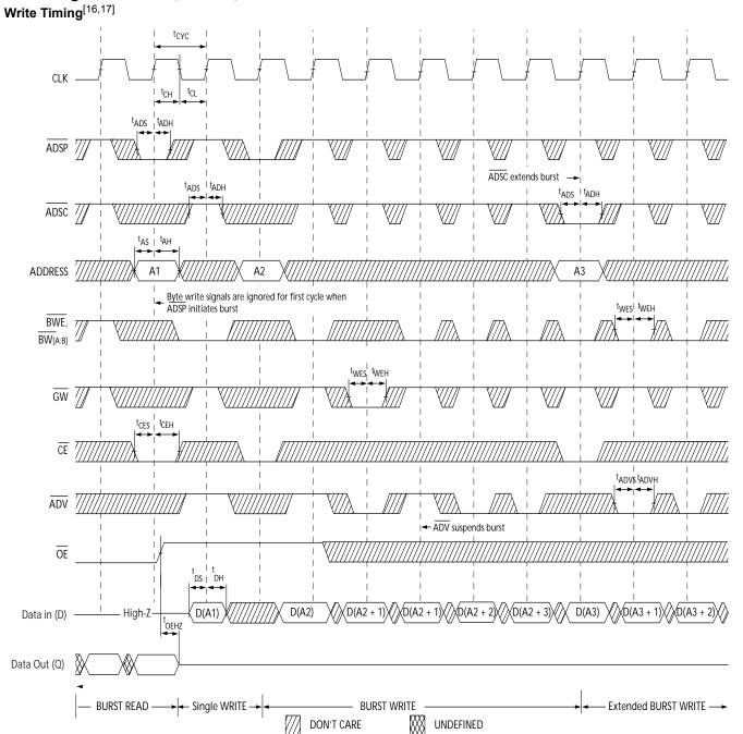
**Note:** 17. Full width write can be initiated by either  $\overline{GW}$  LOW; or by  $\overline{GW}$  HIGH,  $\overline{BWE}$  LOW and  $\overline{BW}_{[A:B]}$  LOW.
