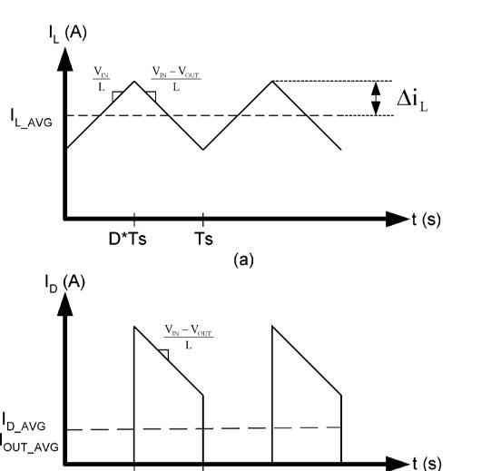
FIGURE 5. (a) Inductor current. (b) Diode current.
