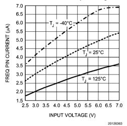
CE Pin Current vs. Input Voltage
