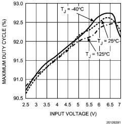
660kHz Max. Duty Cycle vs. Temperature
