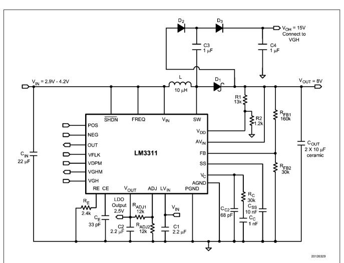
FIGURE 9. Li-lon to 8V, 1.28MHz Application
