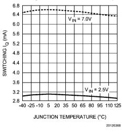
660kHz Switching Quiescent Current vs. Input Voltage
