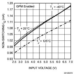
Non-Switching Quiescent Current vs. Temperature GPM Enabled
