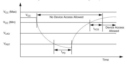
Figure 22. Power-Down or Voltage Drop
