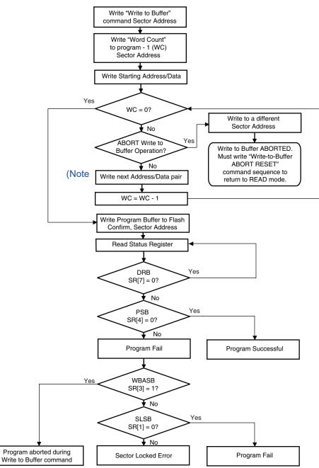
Figure 14. Write Buffer Programming Operation with Status Register
