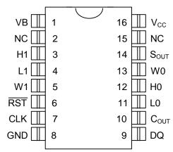
16-Pin SOIC (300-mil) See Mech Orl wings Section
