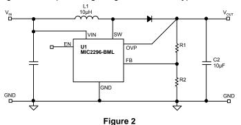
Boost regulation is achieved by turning on an internal switch, which draws current through the inductor (L1). When the switch turns off, the inductor's magnetic field collapses. This causes the current to be discharged into the output capacitor through an external Schottkey diode (D1). Voltage regulation is achieved my modulating the pulse width or pulse width modulation (PWM).
