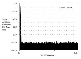
Figure 18. Plot of Ideal 12-bit ADC
