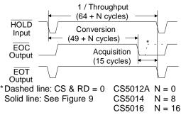
Figure 5b. Synchronous (Loopback Mode)
