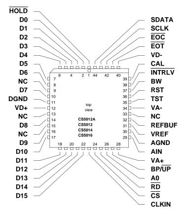
NOTE: All pin references in this data sheet refer to the 40-pin DIP package numbering. Use this figure to determine pin numbers for 44-pin package.
