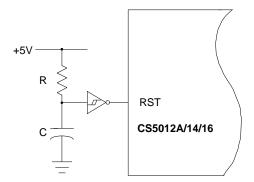
Figure 6. Power-on Reset Circuit
