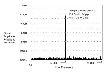
Figure 34. CS5016 FFT plot with 12 kHz -20 dB Input
