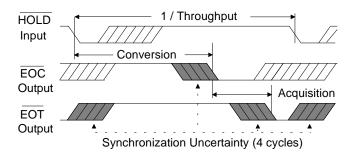
Figure 5a. Asynchronous Sampling (External Clock)
