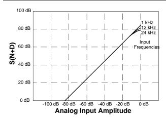
Figure 26. CS5014 S/(N+D) vs. Input Amplitude (9Vp-p Full-Scale Input)
