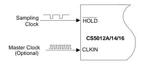
Figure 3a. Asynchronous Sampling
