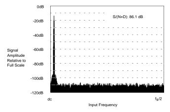
Figure 21. Plot of Ideal 14-bit ADC
