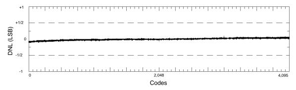
Figure 15. CS5012 Differential Nonlinearity Plot
