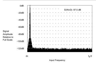
Figure 23. Plot of Ideal 16-bit ADC
