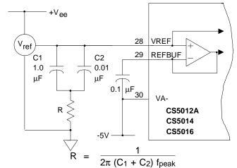
Figure 10. Reference Connections
