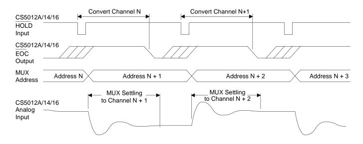
Figure 12. Pipelined MUX Input Channels
