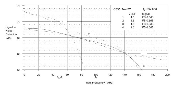
Figure 25. CS5012A High Frequency Input Performance
