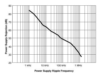
Figure 13. Power Supply Rejection
