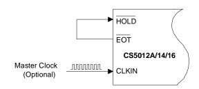
Figure 3b. Synchronous Sampling
