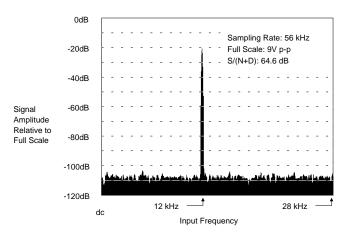
Figure 32. CS5014 FFT plot with 12 kHz -20 dB Input
