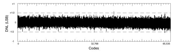
Figure 17. CS5016 Differential Nonlinearity Plot
