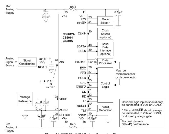
Figure 36. CS5012A/14/16 System Connection Diagram
