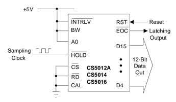
Figure 8. Microprocessor-Independent Connections
