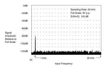
Figure 29. CS5016 FFT plot with 1 kHz -80 dB Input
