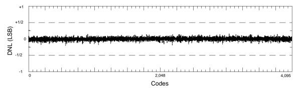
Figure 14. CS5012A Differential Nonlinearity Plot
