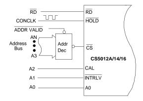
Figure 4a. Conversions Asynchronous to CLKIN
