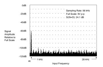
Figure 27. CS5014 FFT plot with 1 kHz -60 dB Input
